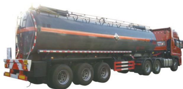
3 axles 56CBM liquid chemical tank semi trailer
