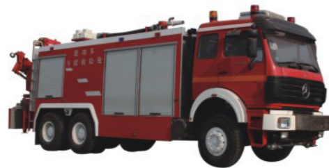
North Benz, Engine 340hp, Volume: 10-12m3
