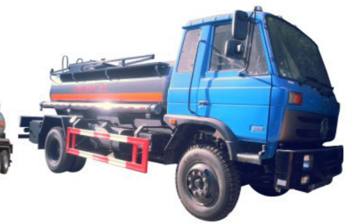
Dongfeng 4x2 chassis, 190 hp , 10cbm chemical tank for caustic soda
