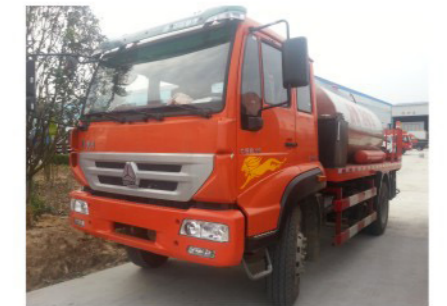
Sinotruk 9-10m3, 190HP Asphalt distribution truck
