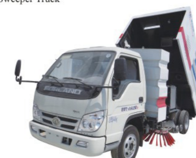
Foton 1.5 water tank & 3-4 m3 dust tank
