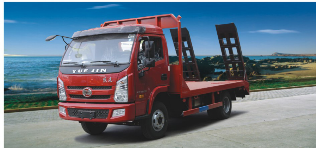
Yuejin Self loading truck (90HP-130HP,6-8 tons,flatbed length:4.7m )
