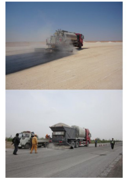
Howo 6*4 asphalt distribution truck, 10m3-12m3, Intelligent automatic control/ half automatic control
