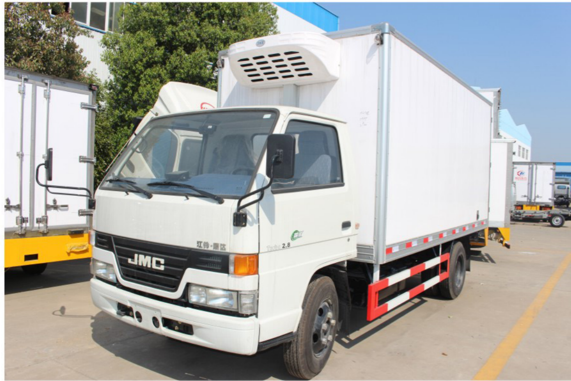
JMC 4x2 Refrigerator truck 3-5tons Engine: 108hp with Euro IV standard Low temperature:-18℃ Refrigerator units:Carrier,Thermo king and more different brands for choose
