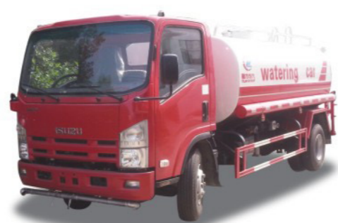
ISUZU water tank truck,engine:ISUZU 190hps, volume:6-8CBM
