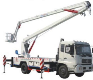
Brand :Dongfeng 4*2 LHD Engine : 160HP ,180HP ,185HP Working Height :18-24m
