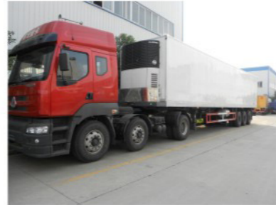
3 axles 40 feet Refrigerator trailer with Carrier units
