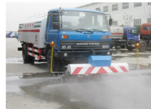
Dongfeng road flushing truck, 8m3 tank, 170hp
