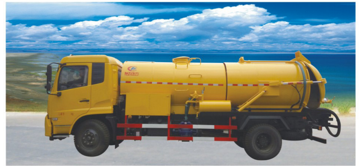
DONGFENG sewer dredging vehicle, 4m3 water tank and 4.5m3 sewage tank, 180hp, cummins engine
