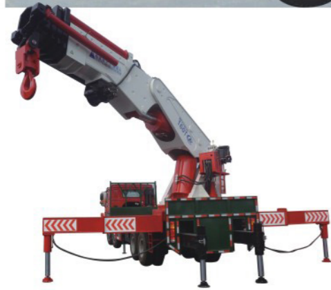
heavy duty truck mounted crane (rear side )
