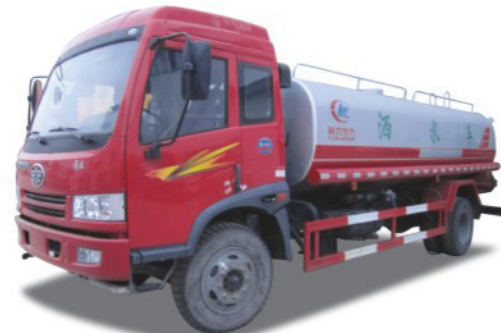
FAW water tank truck, engine:Xichai 180hps, volume:8-10CBM
