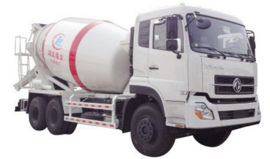
Brand: Dongfeng 6*4 LHD, Engine: 340HP, 375HP Volume: 8cubic meter to 12cubic meter
