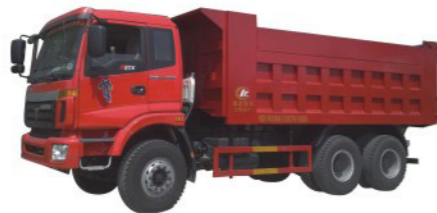
Brand:FOTON 6*4 LHD/RHD Engine: 340HP, 350HP, 380HP Loading Capacity:20T - 35T
