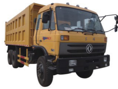
Brand:DONGFENG 6*4 LHD/RHD Engine: 210HP,260HP Loading Capacity:15T - 30T
