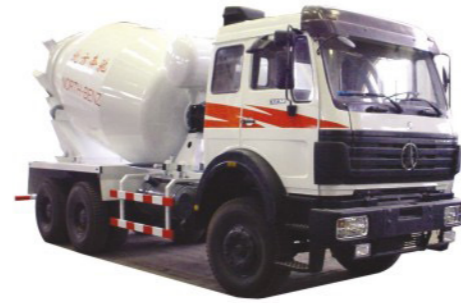
Brand: North Benz 10-12 m3 concrete mixer truck,380HP
