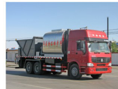
HOWO 6*4 synchronous chip sealer 8m3 asphalt tank+12m3 chip tank
