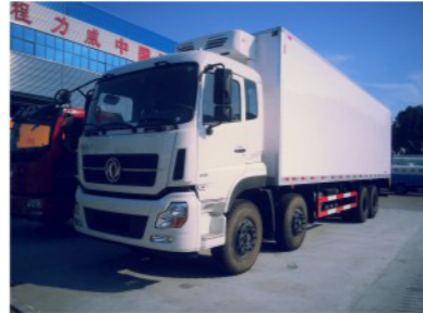
Dongfeng 8x4 Refrigerator truck 30tons
