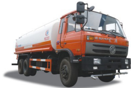
Dongfeng water tank truck, engine:Cummins 210hps, volume:18-20CBM
