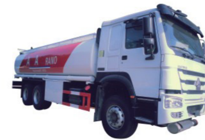
Howo 6x4 chassis, 266 hp , 25-30cbm fuel tank
