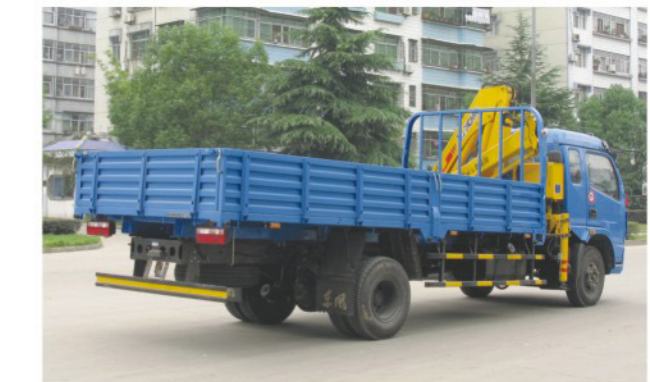
Dongfeng 4x2 truck mounted holding arm crane (2tons to 6tons )
