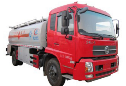
Dongfeng 4x2 chassis, 180 hp , 12-15cbm fuel tank, fuel tank truck
