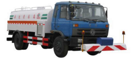
Dongfeng road flushing truck, 8m3 tank, 170hp
