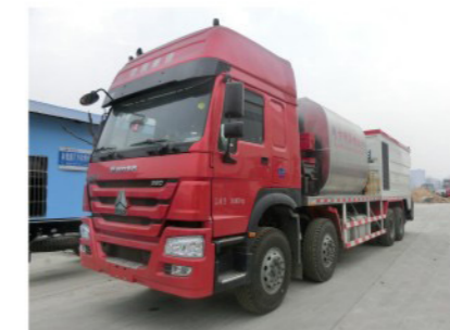
HOWO 8*4 synchronous chip sealer 10m3 asphalt tank+16m3 chip tank
