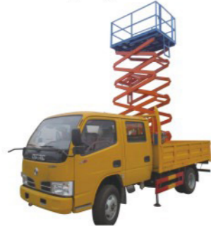
Brand : Dongfeng 4*2 LHD or RHD Engine : 95HP Working Height :6-12m
