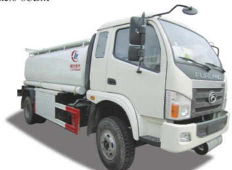
Forland water tank,engine:Yunnei 130hps, volume:8CBM
