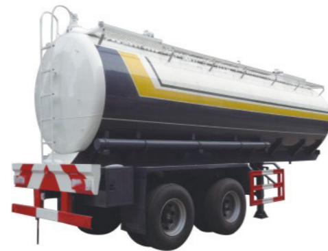
2 axles 40CBM liquid chemical tank semi trailer
