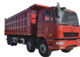
Brand:CAMC 8*4 LHD/RHD Engine: 340HP, 350HP, 380HP Loading Capacity:35T - 45T
