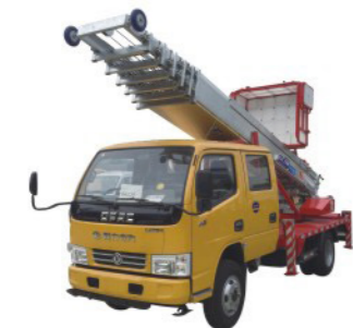
Brand : Dongfeng 4*2 LHD or RHD Engine : 95HP Working Height :20-28m
