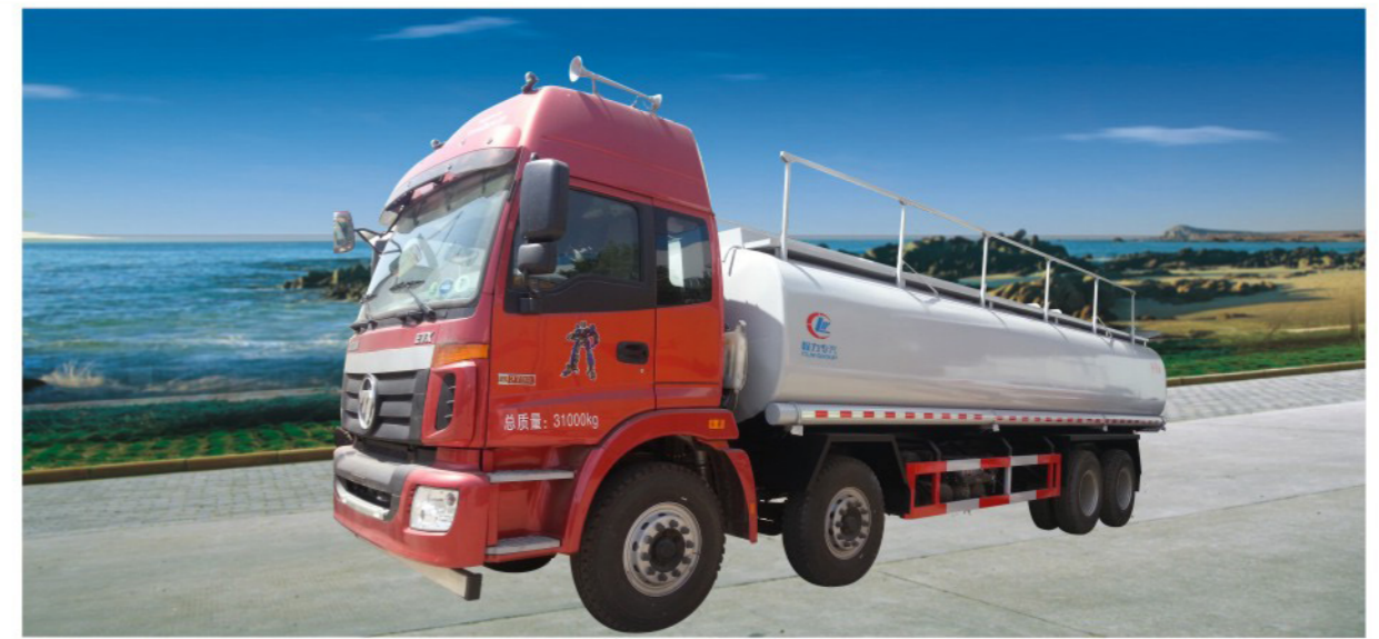
FOTON 8x4 chassis, 290 hp , 30-35cbm fuel tank
