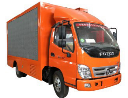
FOTON, Engine: 141hp, LED Screen: Three Sides P8
