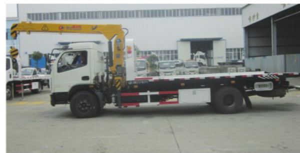
Dongfeng 4x2 wrecker truck mounted crane (2tons to 4tons )
