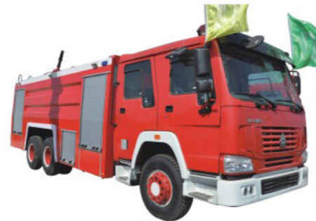
Sinotruk, Engine 336_371hp, Volume: 16m3
