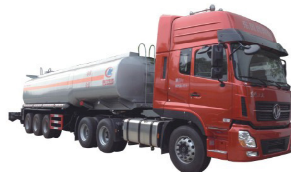
3 axles 48CBM fuel tank semi trailer
